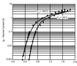
V<sub>SD</sub> – Source-to-Drain Voltage (V)
